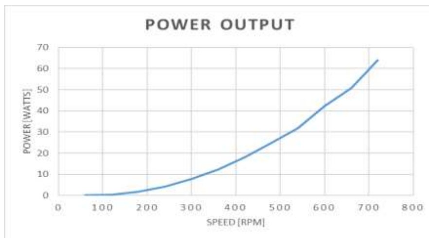
Figure 7. The rectifier power output at different shaft speeds.
