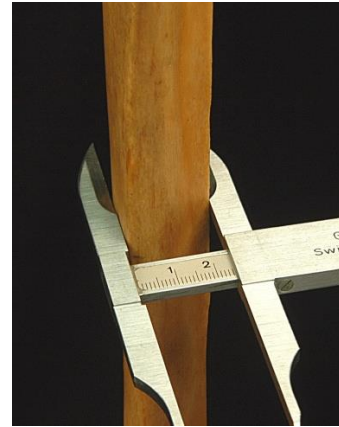
Figure 5. Calipers demonstrating measurement of the anterior-posterior diameter at the midshaft (Langley et al., 2016).
