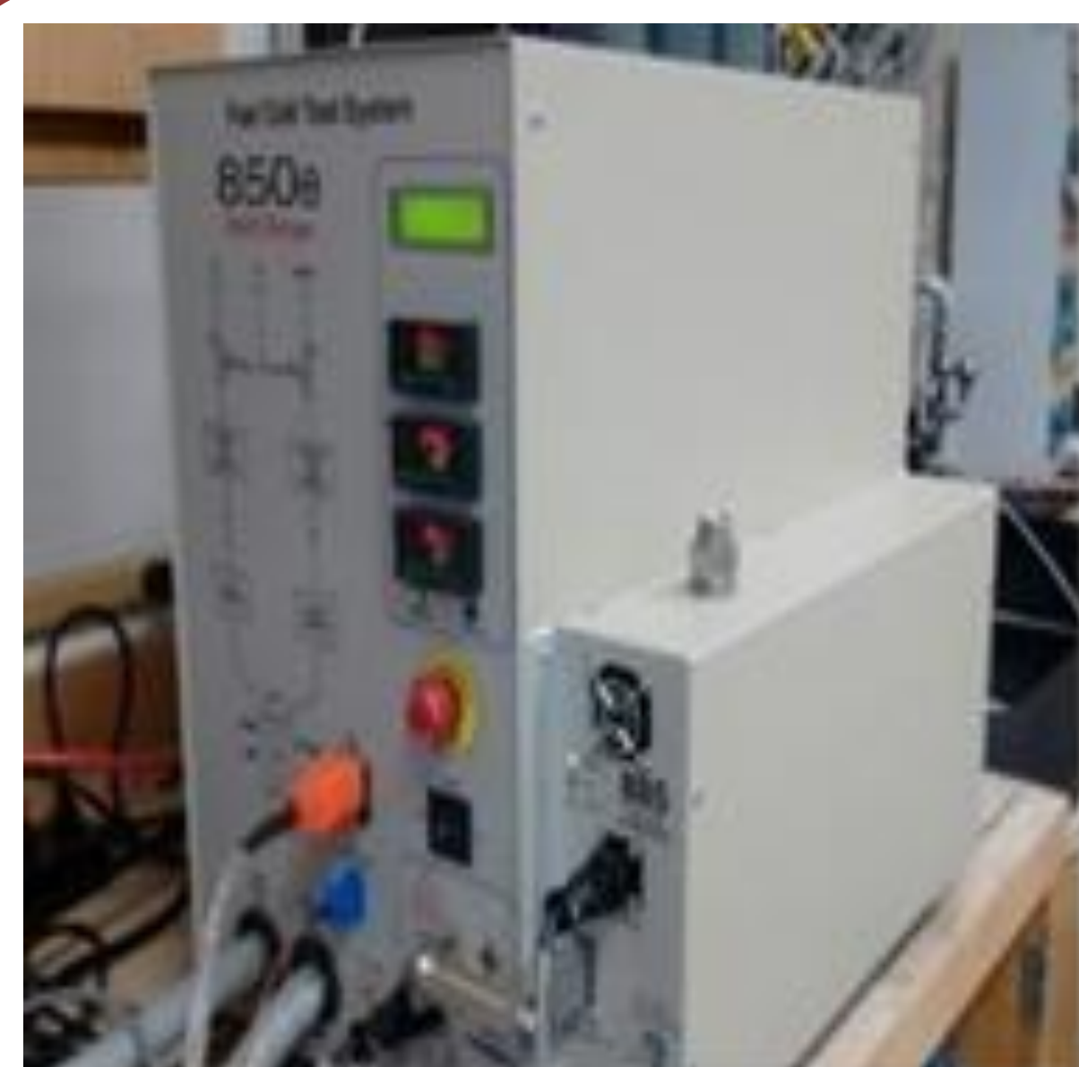
Scribner Associates Inc. 850e Fuel cell system, Assembled BT-112 conductivity cell, and inside view of BT-112 conductivity cell with NCGM coated Nafion 212.
