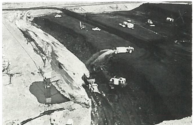
FIGURE 5 Because Wyoming's thick coal seams must be strip mined in 20-30 foot lifts like these in the Big Horn No. 1 mine, a single tipple or delivered sample seldom reflects the composition of the entire seam.
