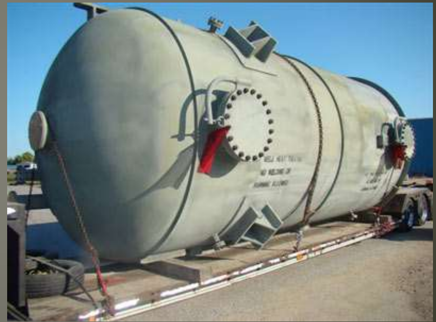
Commercial grade flash drum
