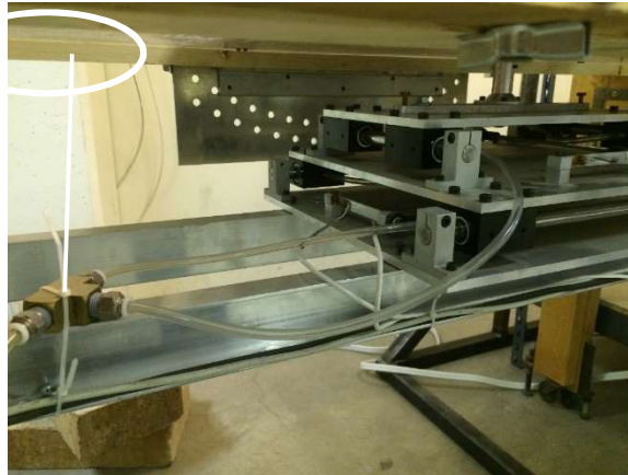
Figure 11. Image of drag and lift measurement apparatus.
