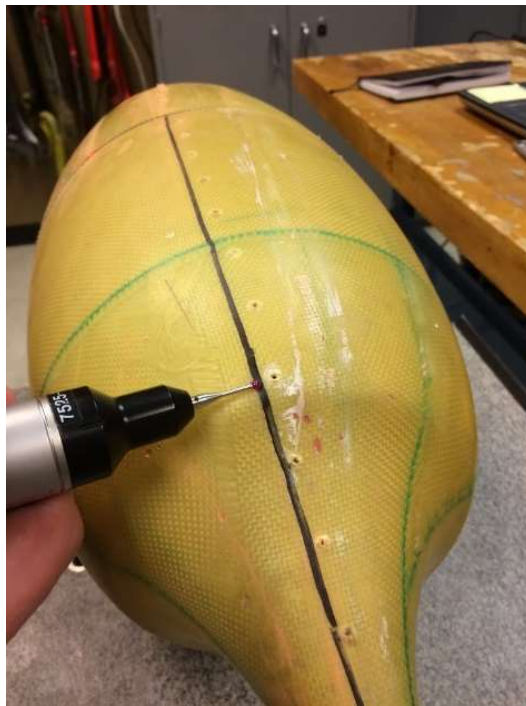
Figure 3. Use of CMM along pre-defined profile line.
