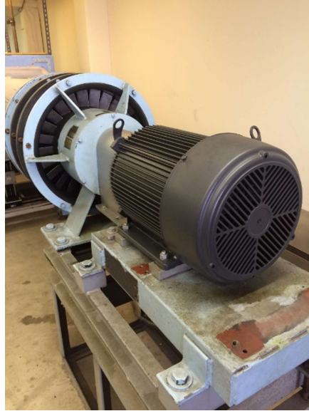
Figure 13. Image of blower used to create flow.
