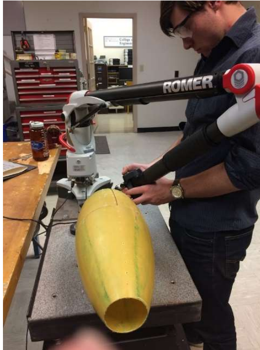
Figure 2. Use of CMM to create a profile of original design.
