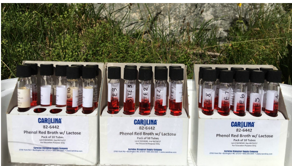
Figure 4: Phenol red lactose broth test tubes with E. coli water samples in them
