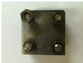
Figure 1. Press cell for making the sample in a pressed condition during the heat treatment.
