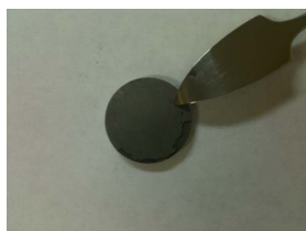
Figure 2. The disk-shaped sample obtained after annealing in hydrogen ambience.
