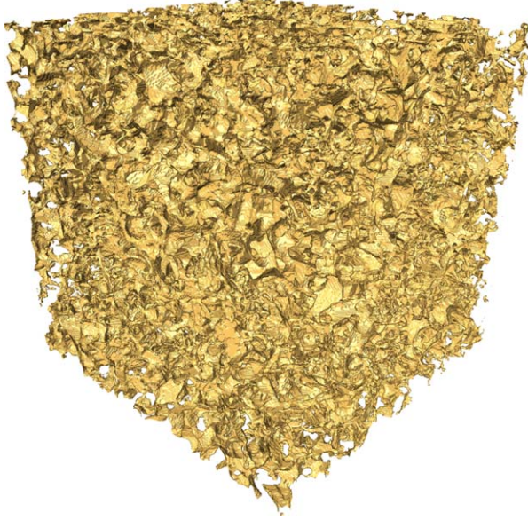
Figure 2. A (2.138 \text{ mm})^3 isosurface of Berea sandstone at 5.345 \text{ }\mu\text{m} resolution.
