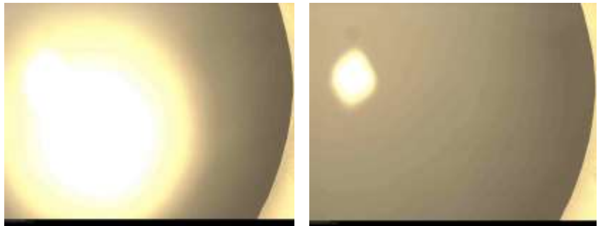
Figure 5: (left) sample image of unfrozen drop from the microscope (right) sample image of frozen drop from the microscope.
