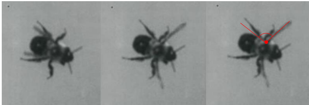
Figure 5: Stroke amplitude. This is the angle measured from the tip of the forewing on the up-stroke to the tip of the forewing on the down stroke.
