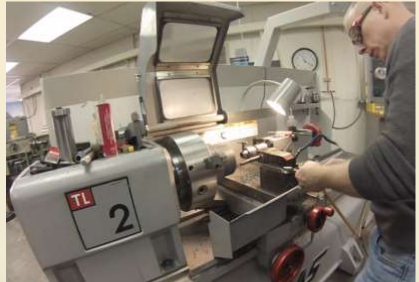
Figure. Shop technician machining compaction cup on CNC Lathe
