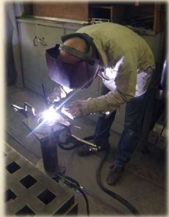
Figure. Technician welding support rings to 4" compaction chamber
