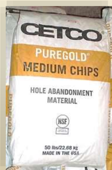
Figure. Raw bentonite
