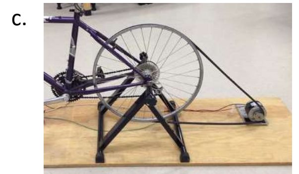
Figure 1: (a) bottle cap generator (Chicargobike, 2010), (b) Atom charger (Siva, 2015), (c) wheel-belt system (DIY Bike Generator, 2015)
