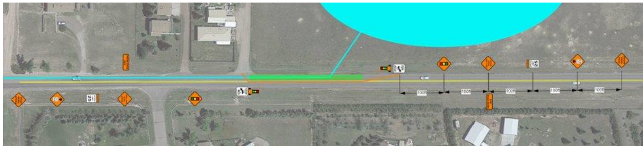
Figure 28: Typical TTC Setup
