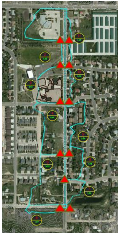
Figure 16: Inlet Location Along Van Buren Ave.
