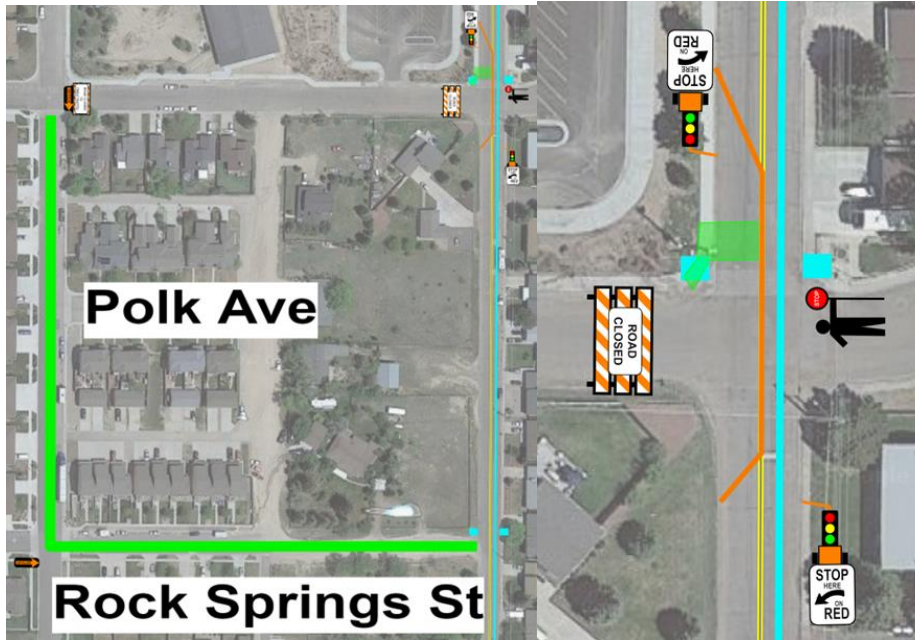
Figure 38: Green River Street (West) TTC and Detour
