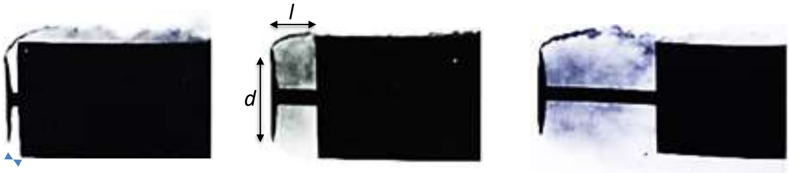
Figure 5. Flow characteristics for bodies in tandem (side view) adapted from Morokin, M.V. N.d. Aerodynamic drag mechanisms of bluff bodies and road vehicles. General discussion and outlook for the future . New York – London: Plenum Press, 1978. 259-260.
