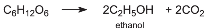
Figure 10. Alcoholic fermentation reaction converting one mole of glucose into two moles of ethanol and two moles of carbon dioxide.
