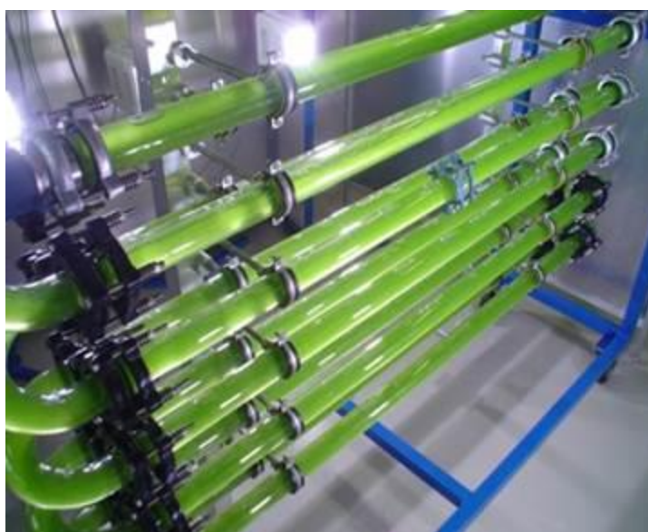
Figure 5. An industrial size photobioreactor
