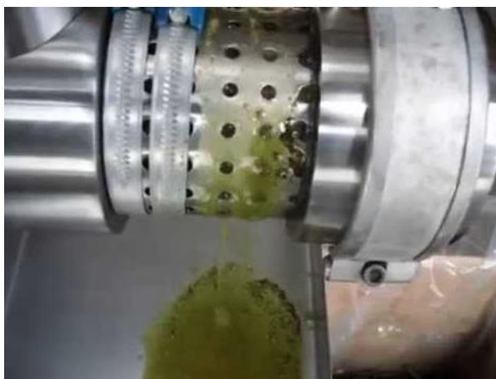
Figure 6. Example of a mechanical algae press for lipid extraction
